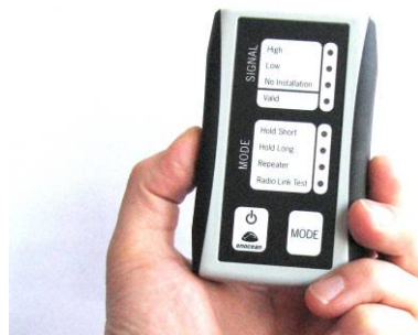
Figure: Field intensity meter EPM 300
