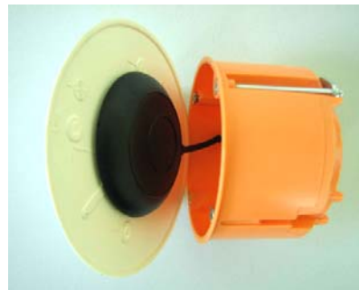
Figure: Mounting a Patch Antenna
