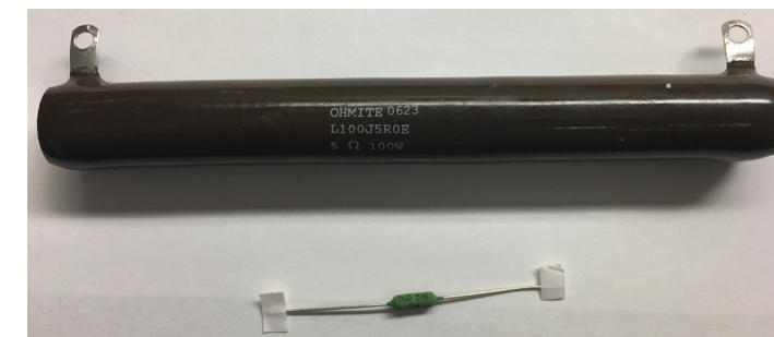
Figure 14: A 100 watt wire element resistor contrasted with one rated for 1 watt.
