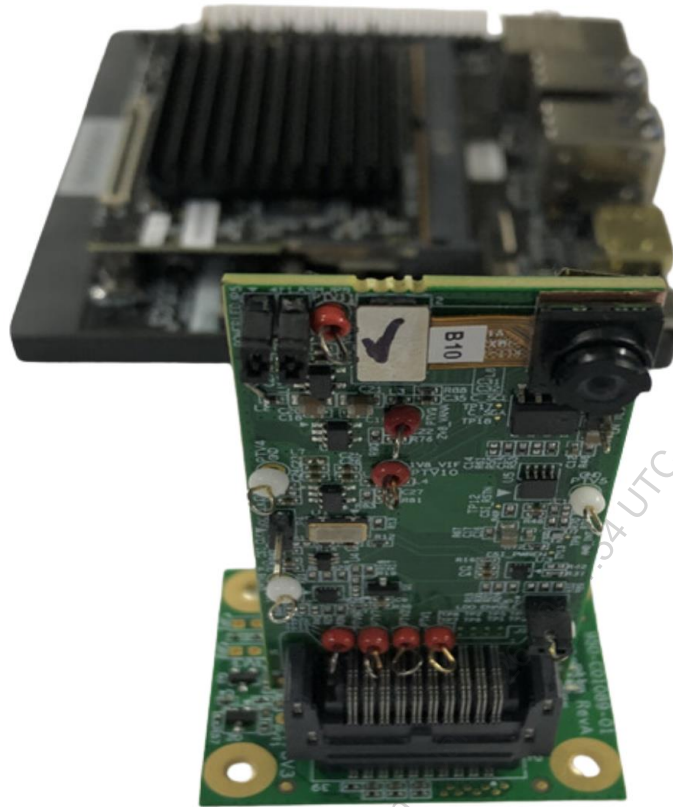
Figure 9. Connector connection with IMX258 module adapter
