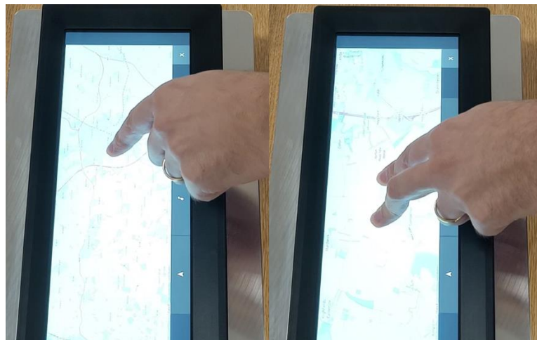
Automotive infotainment system in navigation mode demonstrating one finger push to zoom in, two finger push to zoom out with the rate of zoom being force-dependent
